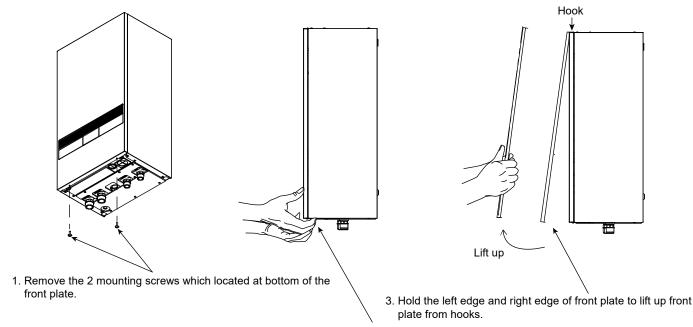
2. Gently pull the lower section of the front plate towards you to remove the front plate from left and right hooks.
