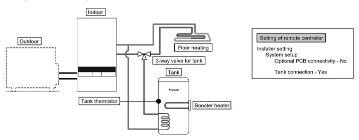
This is an application that connects the DHW tank to the Indoor Unit through 3-way valve. DHW tank's temperature is detected by tank thermistor (specified by Panasonic).
