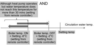
In Advanced Parallel mode, setting for both heating and tank can be made simultaneously. During operation of "Heating/Tank" mode, when each time the mode is switched, the boiler output will be reset to OFF. Please have good understanding on the boiler control characteristic in order to select the optimal setting for the system.
