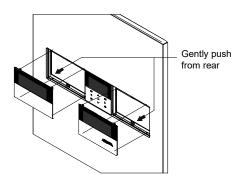
2. Remove the 4 screws and take out the holder with Remote Controller (3).
