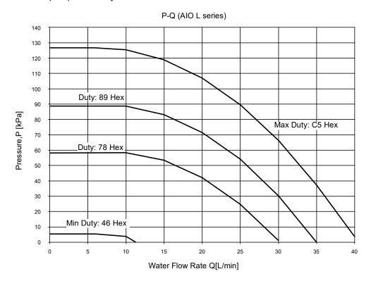
\* This condition is under connecting ODU and connecting 5m piping (inner diameter Φ25) between ODU and IDU (AIO).
