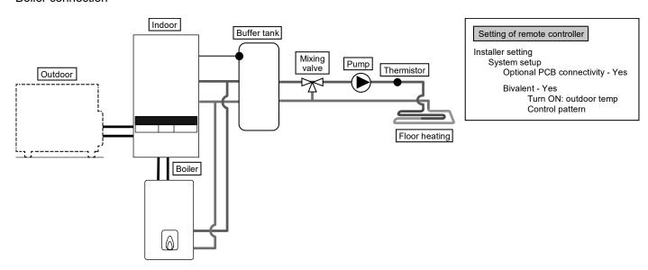
This is an application that connects the boiler to the Indoor Unit, to compensate for insufficient capacity by operate boiler when outdoor temperature drops & heat pump capacity is insufficient.
