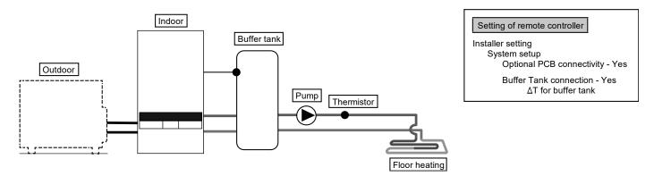
This is an application that connects the buffer tank to the Indoor Unit. Buffer tank's temperature is detected by buffer tank thermistor (specified by Panasonic). This system requires Optional PCB (CZ-NS5P).
