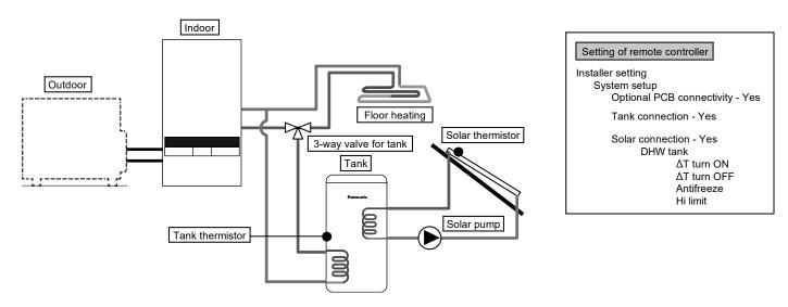
This is an application that connects the DHW tank to the Indoor Unit through 3-way valve before connect the solar water heater to heat up the tank. DHW tank's temperature is detected by tank thermistor (specified by Panasonic). Solar panel's temperature is detected by solar thermistor (specified by Panasonic).
