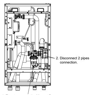
Turn to remove the Magnet Bar at bottom of Magnetic Water Filter Set.
