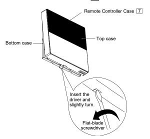
3. Reverse the steps 1 to 4 of section "Remove The Remote Controller From Indoor Unit" to fix Remote Controller Case 7 on Indoor Unit.
