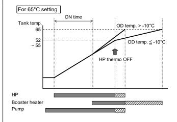
Internal A setting which is using backup heater of Indoor Unit to boil the tank.
