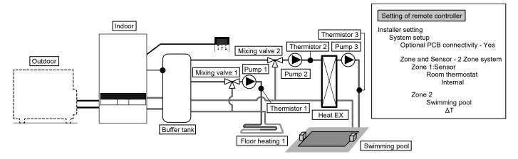
Connect floor heating and swimming pool to 2 circuits through buffer tank as shown in figure.
