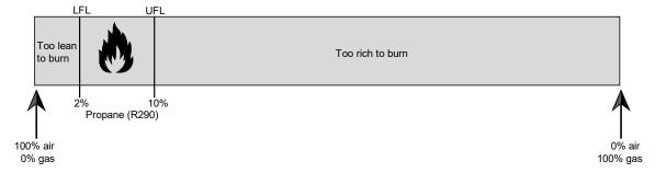
The concentration of R290 between the lower flammable limit (2%) and upper flammable limits (10%) is enough to ignite fire.
