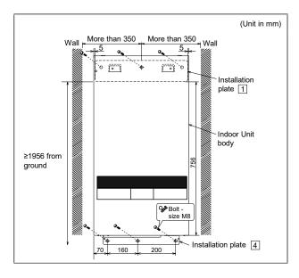
The centre of installation plate should be at more than 350 mm at right and left of the wall.
