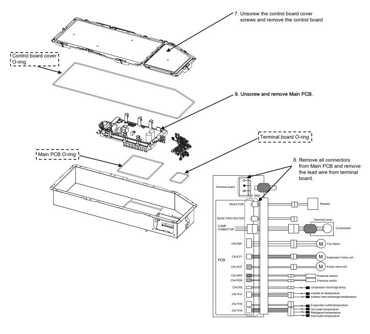
Note: During re-assemble the Main PCB, ensure to attach the O-ring properly to avoid gas leakage into the control board complete.
