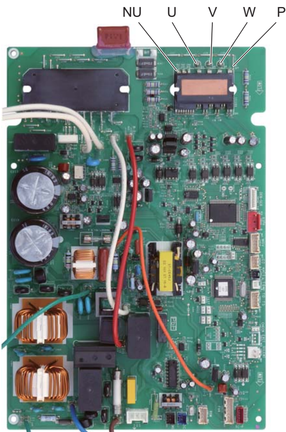
■ Outdoor Unit Control PCB CR-60PEY1E5 : bottom (U-60PEY1E5) (for single-phase outdoor unit PCB)
