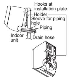
There is an option to use the holder at the rear of chassis to prop up the indoor unit as shown in the illustration for ease of installation. Push the holder back to original position before secure the indoor unit.
