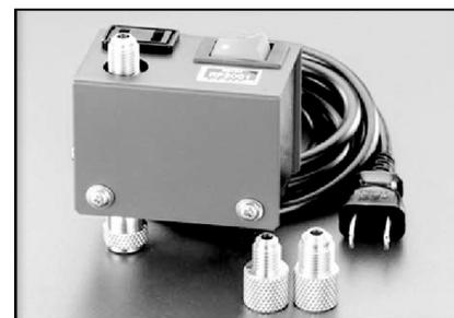
7. HFC refrigerant\_Electric gas leakage tester
