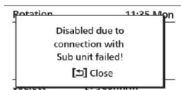
Please ensure that both CNT cables are connected properly at indoor unit and wired remote controller according to CNT cable Installation Manual. After that, repeat Steps 1. to 5. (Contact an authorised dealer if problem persists).
