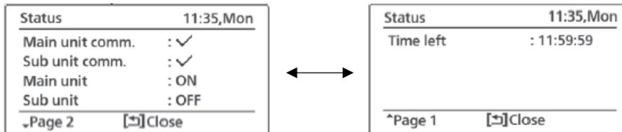
b. **Rotation Status** screen during Duty Rotation = ON with communication error only:
