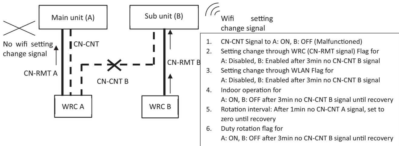
E) During Duty Rotation = ON, both CN-CNT A and B are malfunctioned
