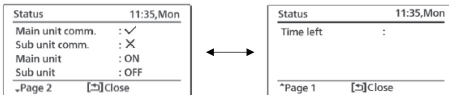
c. **Rotation Status** screen during Duty Rotation = ON with system error only:
