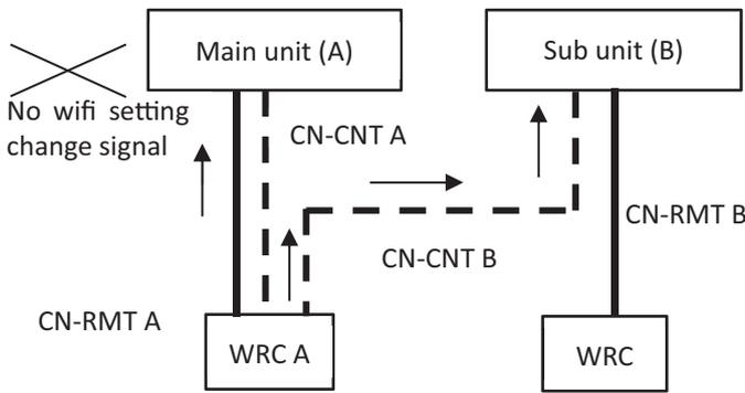
1. CN-CNT Signal to A and B: ON
