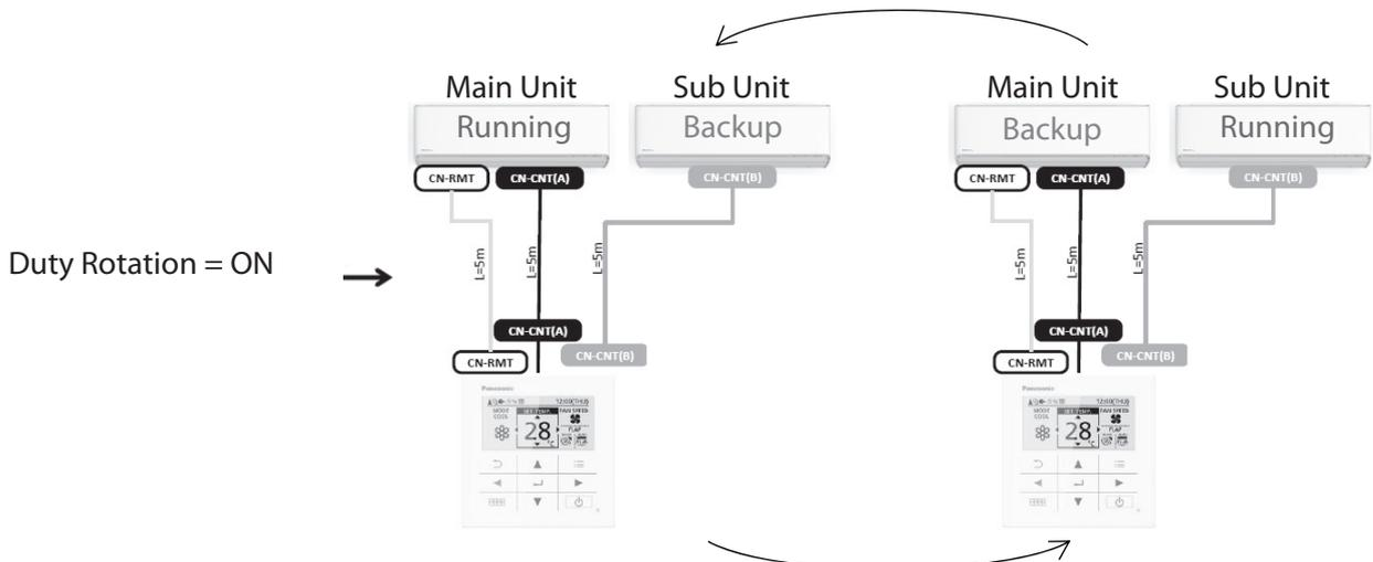
2. After rotation interval ends, Main unit will be turned off (becomes backup unit) and Sub unit will be turned on (becomes running unit) for the next rotation cycle. Role of running and backup unit will rotate between Main and Sub unit for each new rotation cycle.
