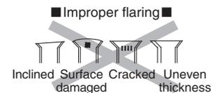
When properly flared, the internal surface of the flare will evenly shine and be of even thickness. Since the flare part comes into contact with the connections, carefully check the flare finish.
