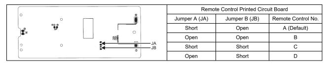
During Remote Control Number Switch Mode, press any button at remote control to transmit and store the transmission code to the EEPROM. 4 REMOTE CONTROL RECEIVING SOUND OFF/ON MODE
