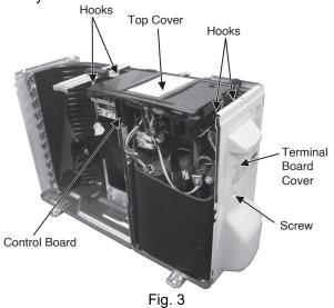
5 Remove the Control Board as follows:
