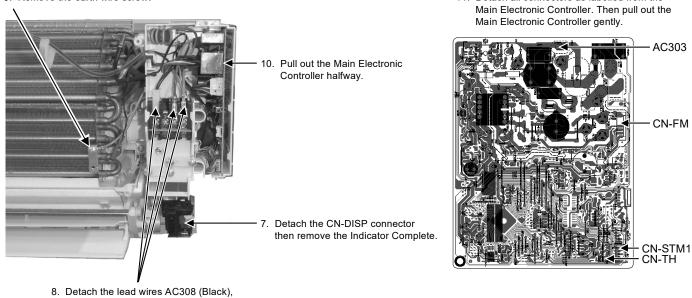
. Detach the lead wires AC308 (Black), AC307 (Brown), AC304 (Red) and G301 (Green) from the Terminal Board.
