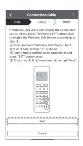
. Ensure Wireless LAN LED is ON. Press and hold the Wireless LAN 🕏 button for 5 seconds until "1" is shown on the remote control and press 🗊 pointing to the air conditioner.
