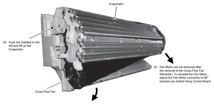
21. Remove the Cross Flow Fan from the unit by pulling it to the left and downward.
