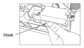
2 Remove the cover by unclipping it and pulling it out.
