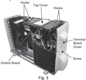
Remove the Control Board as follows:
