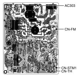
Detach the lead wires AC308 (Black), AC307 (Brown), AC304 (Red) and G301 (Green) from the Terminal Board.
