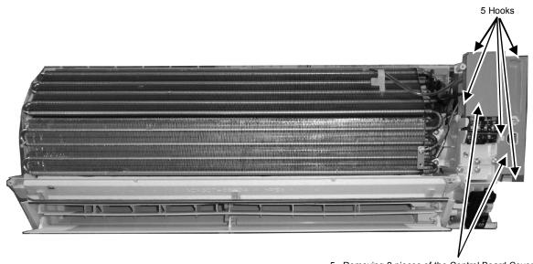
5. Removing 2 pieces of the Control Board Cover by releasing the 5 hooks.
