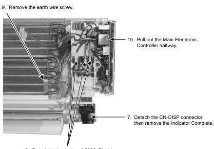
Detach all connectors as labelled from the Main Electronic Controller. Then pull out the Main Electronic Controller gently.
