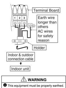
Earth wire shall be Yellow/Green (Y/G) in colour and longer than other AC wires for safety reason.
