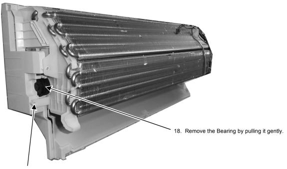
17. Remove the screw from the Evaporator.
