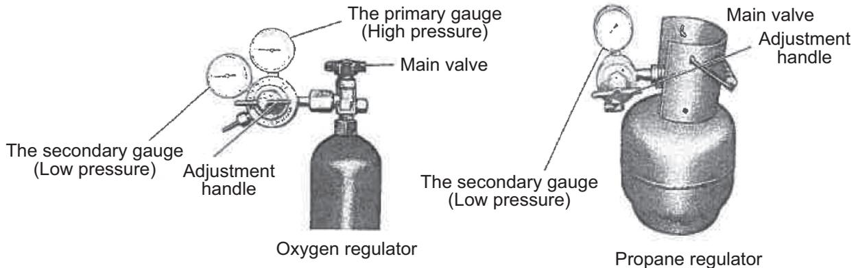
2. Open the cylinder valve, and check the remaining amount with the first side pressure gauge.
