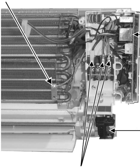
10. Pull out the Main Electronic Controller halfway.
