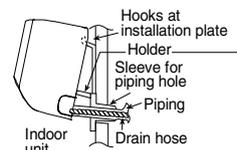
There is an option to use the holder at the rear of chassis to prop up the indoor unit as shown in the illustration for ease of installation. Push the holder back to original position before secure the indoor unit.
