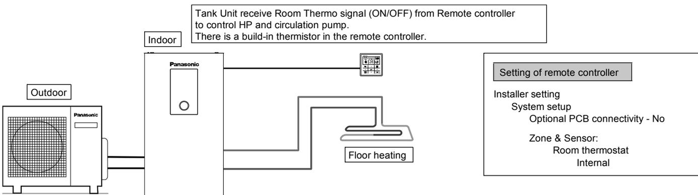
Connect floor heating or radiator directly to the Tank Unit.
