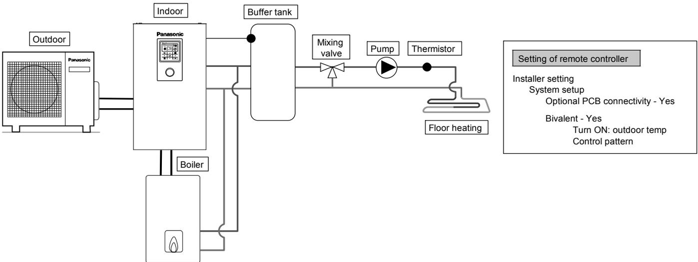
This is an application that connects the boiler to the Tank Unit, to compensate for insufficient capacity by operate boiler when outdoor temperature drops & heat pump capacity is insufficient.
