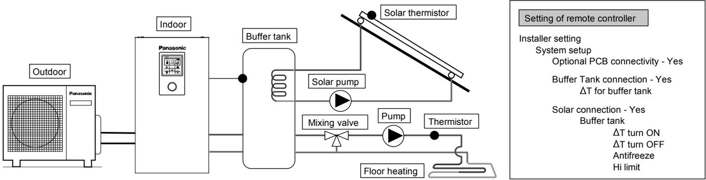
This is an application that connects the buffer tank to the Tank Unit before connecting to the solar water heater to heat up the tank.
