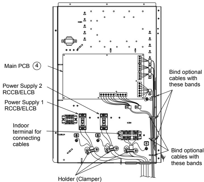
How to guide the optional cables and power supply cord
