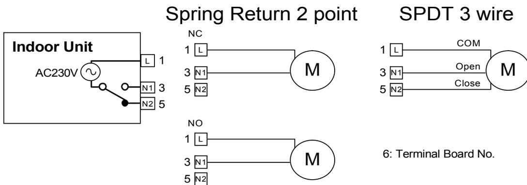
\* During pump down and force mode, fix 3 ways valve in close condition.
