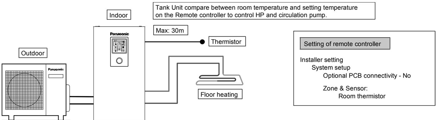
Connect floor heating or radiator directly to Tank Unit.
