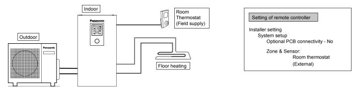
Connect floor heating or radiator directly to Tank Unit. Remote controller is installed on Tank Unit.
