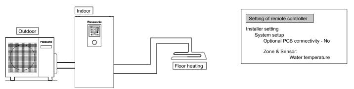
Connect floor heating or radiator directly to the Tank Unit. Remote controller is installed on Tank Unit. This is the basic form of the most simple system.
