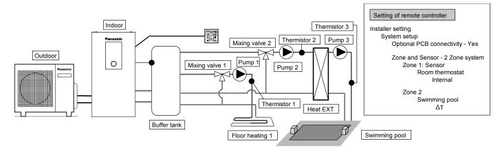
Connect floor heating and swimming pool to 2 circuits through buffer tank as shown in figure. Install mixing valves, pumps and thermistors (specified by Panasonic) on both circuits.
