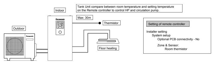
Connect floor heating or radiator directly to Tank Unit.
