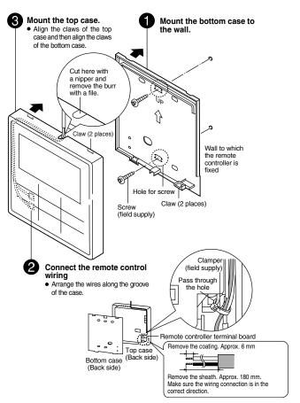
For embedded type **Preparation:** Make 2 holes for screws using a driver.
