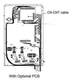
Insert a flat head screwdriver into the slot on the top of the adaptor and remove the cover. Connect the other end of the CN-CNT cable connector to the connector inside the adaptor.
