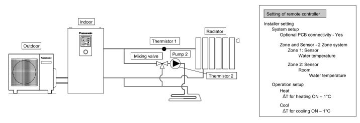
This is an example of simple 2 zone control without using buffer tank.
