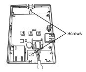
• Pull the CN-CNT cable through the hole in the bottom of the adaptor and re-attach the front cover to the back cover.
