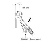
Do not overtighten, overtightening may cause gas leakage.
