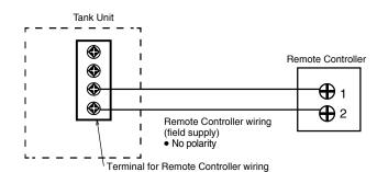
Remote Controller cable shall be (2 x min 0.3 mm<sup>2</sup>), of double insulation PVC-sheathed or rubber sheathed cable. Total cable length shall be 50 m or less.
