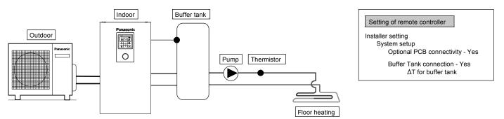
This is an application that connects the buffer tank to the Tank Unit.
