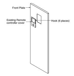
2 Press from front to fix the Remote controller cover on the front plate.
