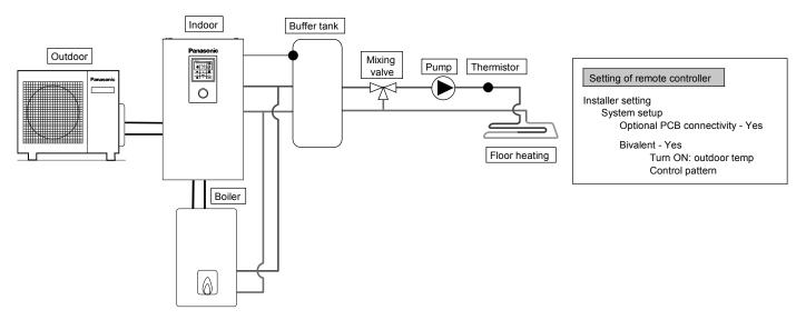
This is an application that connects the boiler to the Tank Unit, to compensate for insufficient capacity by operate boiler when outdoor temperature drops & heat pump capacity is insufficient.
