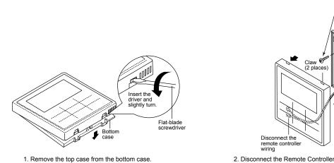
2. Disconnect the Remote Controller wiring.
