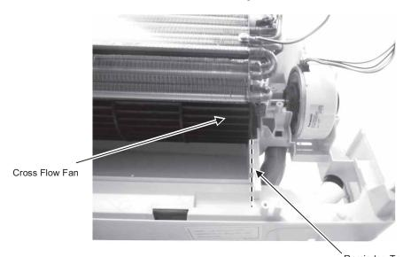
Reminder: To reinstall the cross flow fan, ensure cross flow fan is in line as shown in figure 12.
