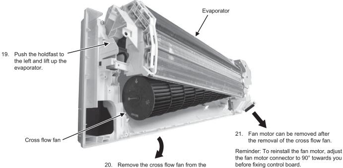
20. Remove the cross flow fan from the unit by pulling it to the left and downward.
