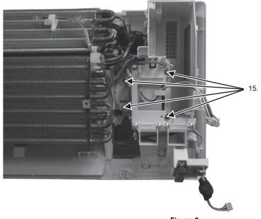
Remove the 4 screws holding the control board, then pull out the control board.
