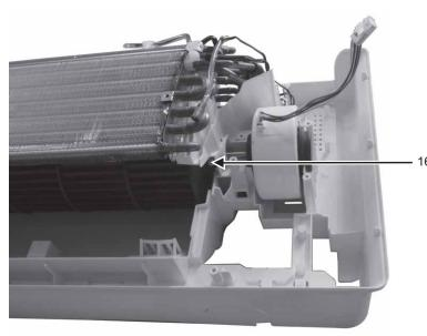
16. Remove the screw that holding the cross flow fan and fan motor axis.
