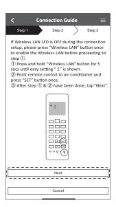
Ensure Wireless LAN LED is ON. Press and hold the Wireless LAN ♀ button for 5 seconds until "1" is shown on the remote control and press ➡ pointing to the air conditioner.
