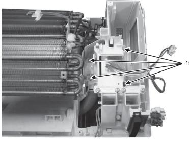
Remove the 4 screws holding the control board, then pull out the control board.
