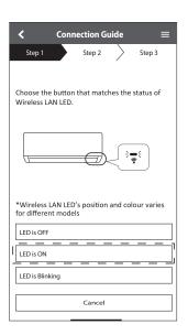
2. When Wireless LAN LED is blinking, select preffered connection setup mode.
