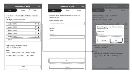
4. Select the SSID of your wireless router. Enter the password to connect the air conditioner to the wireless router.
