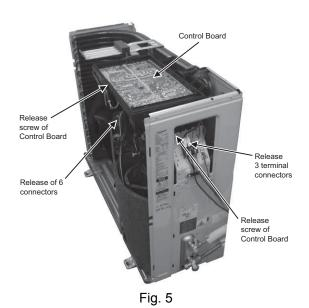
7. Remove the 4 screws of the Electronic Controller.
