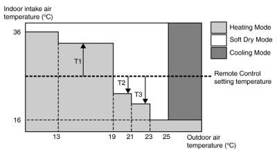
• Every 180 minutes, the indoor and outdoor temperature is judge. Based on remote control setting temperature, the value of T1 will increase up to 10°C, T2 will decrease by 3°C and T3 will decrease up to 8°C.
