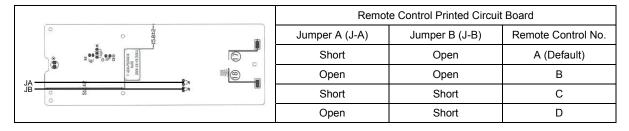
During Remote Control Number Switch Mode, press any button at remote control to transmit and store the transmission code to the EEPROM.
