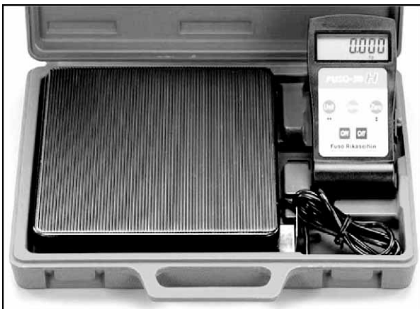
Digital scale for refrigerant charging
