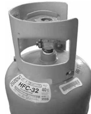
10. Connection ports of refrigerant cylinders and packing
