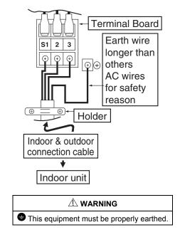
• Earth wire shall be Yellow/Green (Y/G) in colour and longer than other AC wires for safety reason.
