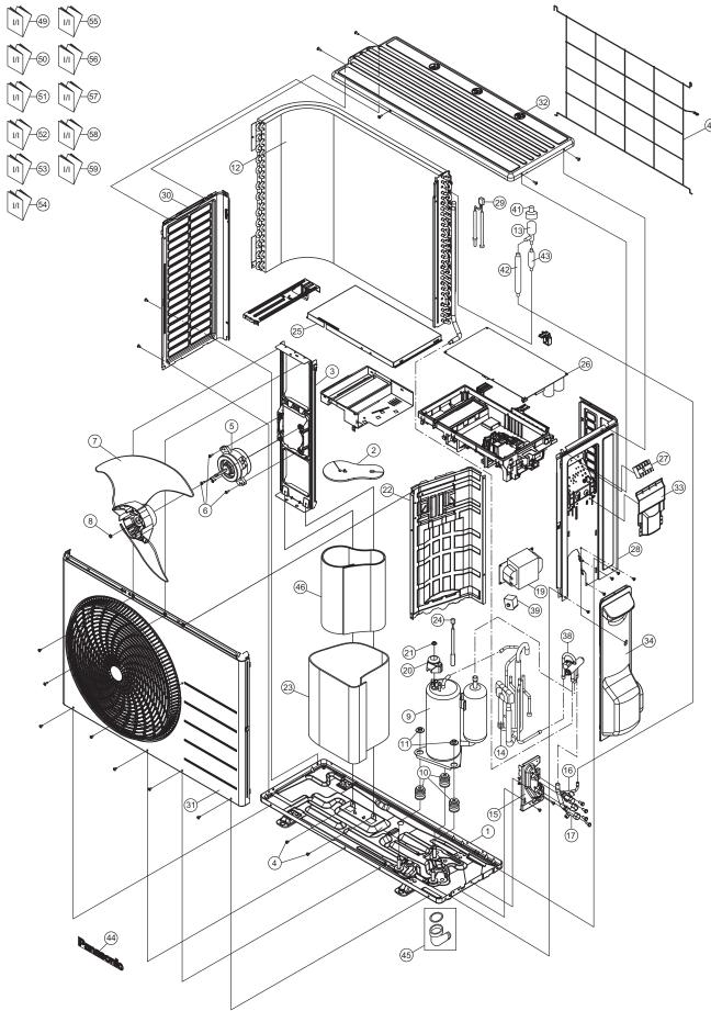
The above exploded view is for the purpose of parts disassembly and replacement. The non-numbered parts are not kept as standard service parts.
