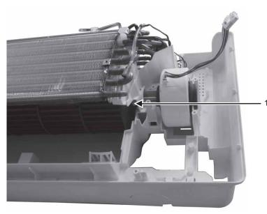
15. Remove the screw that holding the cross flow fan and fan motor axis.
