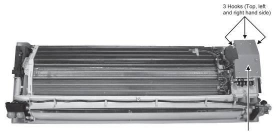
Remove control board cover by releasing 3 hooks.
