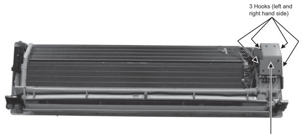
Remove control board cover by releasing 4 hooks.
