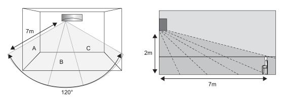
Human Activity sensor will turns on according to infrared sensors signal detection.
