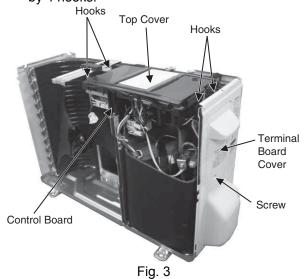
5 Remove the Control Board as follows:
