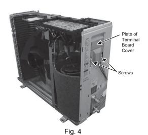
6 Remove the Control Board.
