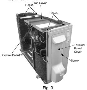
5 Remove the Control Board as follows:
