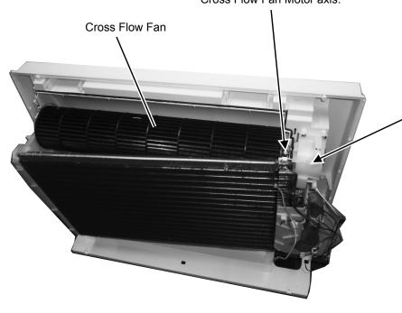
Release the 4 screws of the Fan Motor.
