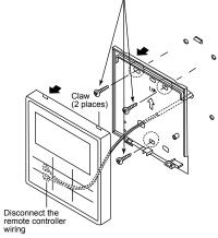
2. Disconnect the Remote Controller wiring.
