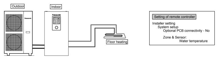
Connect floor heating or radiator directly to the Tank Unit. Remote controller is installed on Tank Unit. This is the basic form of the most simple system.
