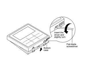
1. Remove the top case from the bottom case.
