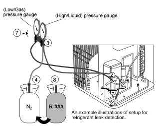
Step 2: Refrigerant leak detection through Electronic halogen leak detector and/or ultrasonic leak detector:
