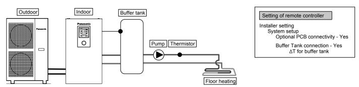
This is an application that connects the buffer tank to the Tank Unit. Buffer tank's temperature is detected by buffer tank thermistor (specified by Panasonic). This system requires Optional PCB (CZ-NS4P).
