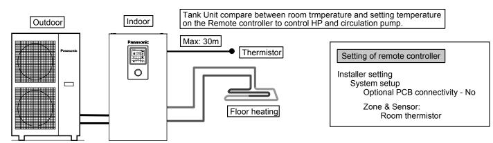
Connect floor heating or radiator directly to Tank Unit.
