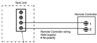
Terminal for Remote Controller wiring
