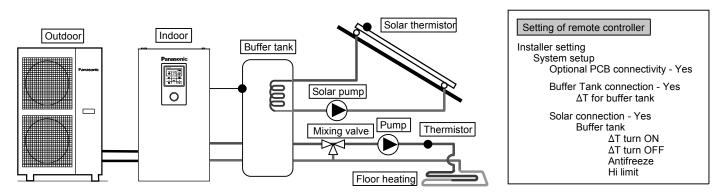
This is an application that connects the buffer tank to the Tank Unit before connecting to the solar water heater to heat up the tank.
