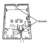
• Pull the CN-CNT cable through the hole in the bottom of the adaptor and re-attach the front cover to the back cover.
