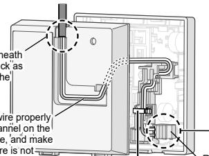
Insert the wire properly into the channel on the bottom case, and make sure the wire is not pinched when the case is attached to the wall.
