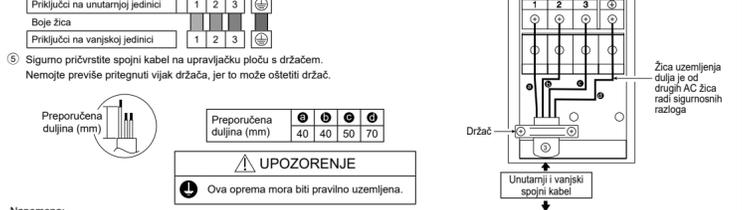
Instructions for connecting the outdoor unit cables, including wire identification and termination points.
